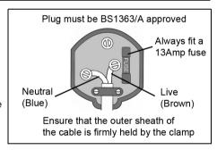
We strongly recommend that this machine is connected to the mains supply via a Residual Current Device (RCD). If you are not sure, consult a qualified electrician.
